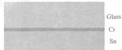
Fig. 9 # 1 specimen Chromium and tin film are deposited sequentially on glass substrate.
